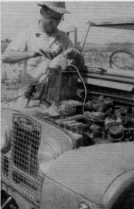
On our way home we have a fuel pump failure. A makeshift arrangement of tin can, plastic bag, and petrol tin meets the emergency.
